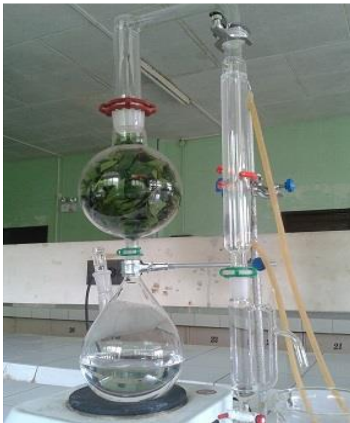
Fig 2: Steam Distillation Setup employed in the experiment
